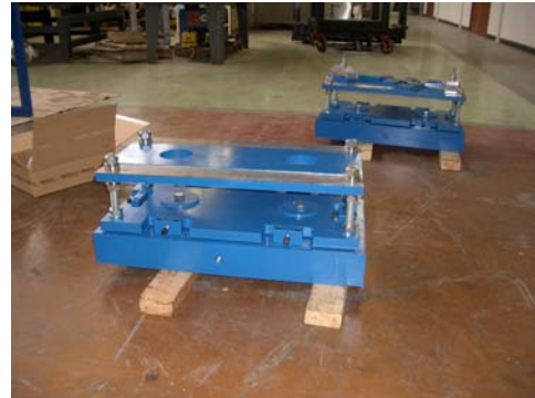
Second Frame support carriage manufactured and assembled by Liverpool University workshops.
